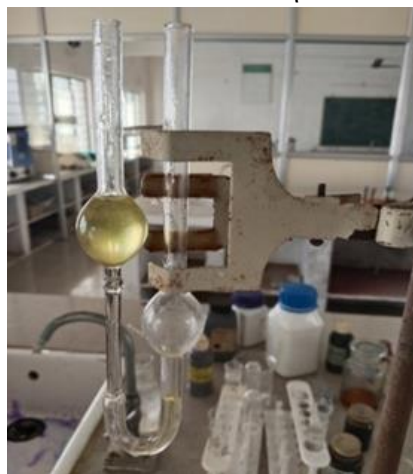
Fig.8 Ostwald Viscometer Contain Kalanchoe Pinnata Leaf Syrup
